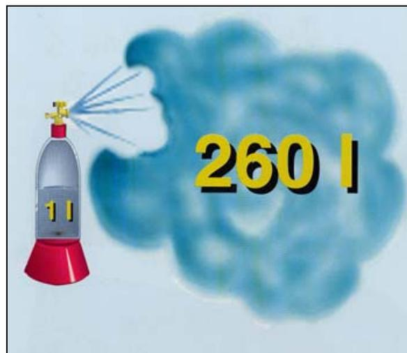
**Figure 2.4:** Evaporation of even small quantities of flammable liquids (such as liquefied propane) may give rise to large quantities of flammable vapours. Note: 1 litre of liquid propane when transformed into gas and diluted in air to the lower explosive limit would give a 13,000 litre explosive atmosphere.<sup>4</sup>
